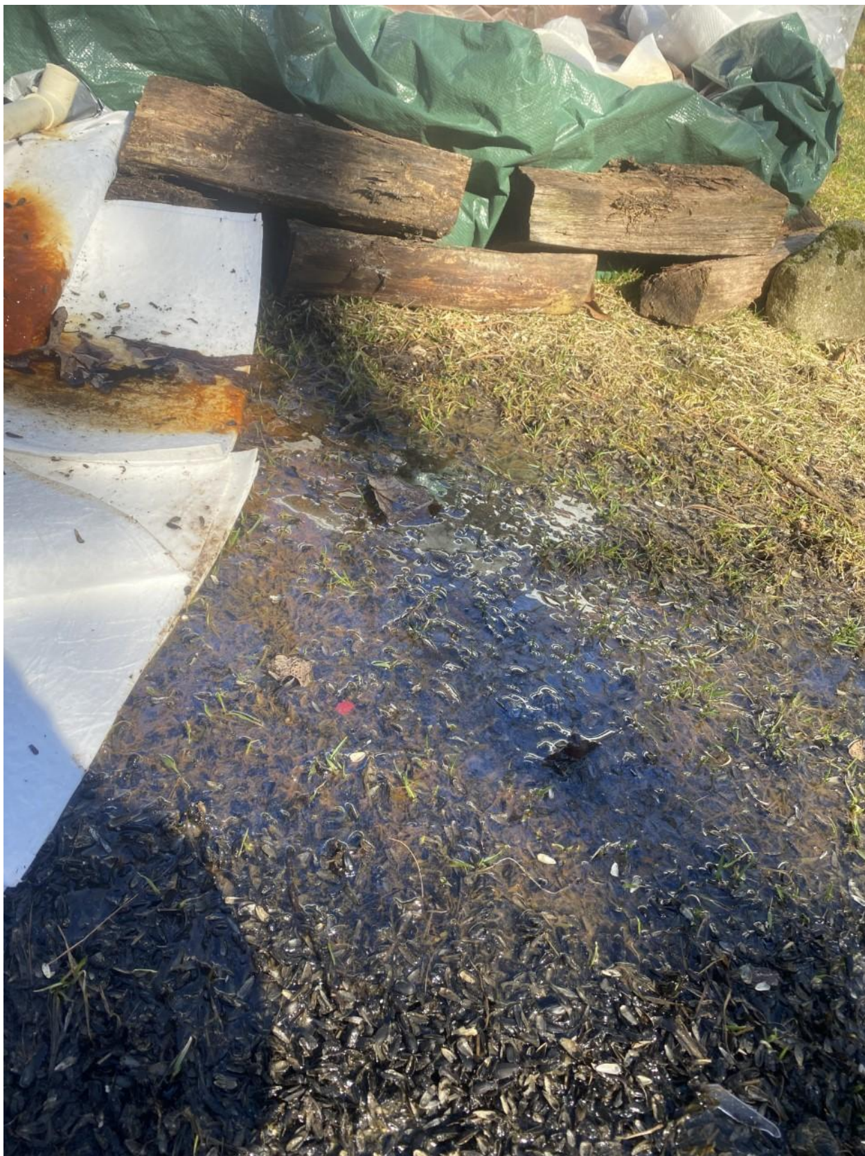
Figure 4. Oil sheen from spill.
