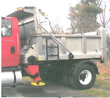
Conveyor uses 667X type pintle chain at 16" wide with 3/8" x 1-1/4" flites on 4-1/2" centers. The conveyor is a self-cleaning drag chain powered through a reducing gearbox and hydraulic motor.
