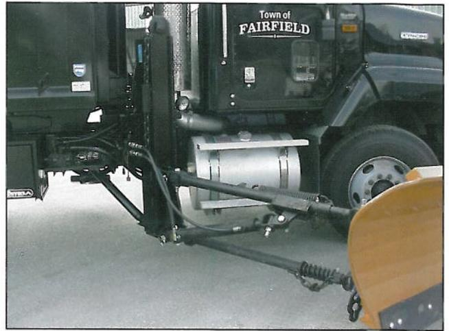
Totally hydraulic rear tower. Completely enclosed rear cabinet with hydraulic cylinder located inside for protection. Tower slider attached directly to cylinder end for positive lift. Square bar slider keeper track full length of rear tower.
